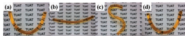
Figure 4. Shape memory properties of 18 wt % (5.2 vol %) surface-modified TiO 2 /epoxy composites. (a) Initial structure, (b) (c) examples of changed shapes, and (d) shape recovery after second heating process. The diameter and length of the composite tube were 4.0 and 100 mm, respectively.
