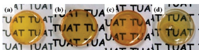
Figure 3. TiO 2 nanoparticles dispersed in epoxy and PMMA resins. (a) 2.4 wt % (0.6 vol %) in epoxy, (b) 13 wt % (3.8 vol %) in epoxy, (c) 18 wt % (5.2 vol %) in epoxy, and (d) 6.4 wt % (1.8 vol %) in PMMA. The diameter and thickness of the pellet were 25 and 2 mm, respectively.
